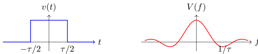
Figure 3.3: A rectangular pulse in time corresponds to an infinite Sinc function in frequency.
