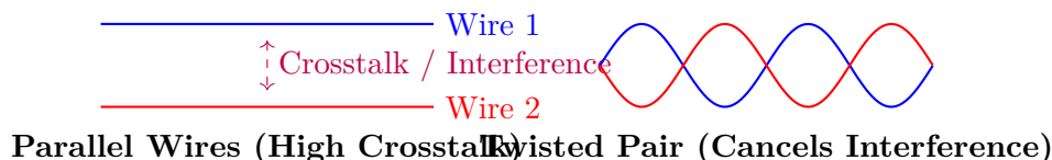
Figure 3.37: The physical twisting of copper wires cancels out Electromagnetic Interference (EMI) and crosstalk.
