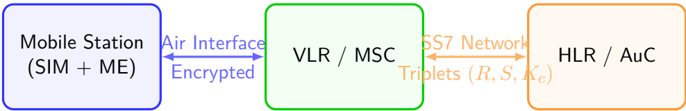
Figure 2.1: Key components interacting in GSM authentication.
