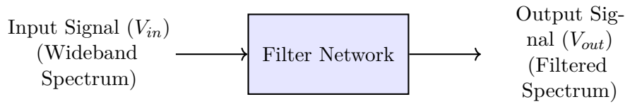
Figure 5.90: Basic Block Diagram of a Filter Operation
