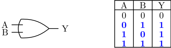
Figure 2.8: The OR Gate symbol and Truth Table.
