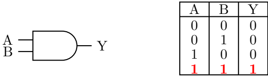
Figure 2.7: The AND Gate symbol and Truth Table. Notice that the output is only '1' in the final row.
