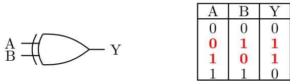
Figure 2.12: The Exclusive-OR Gate. Notice the extra curved line at the input, and the \oplus symbol in the Boolean equation.
